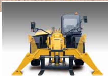
Wide type stabilisers guarantee highest stability on any ground type. Cylinders are well protected inside the frame.
