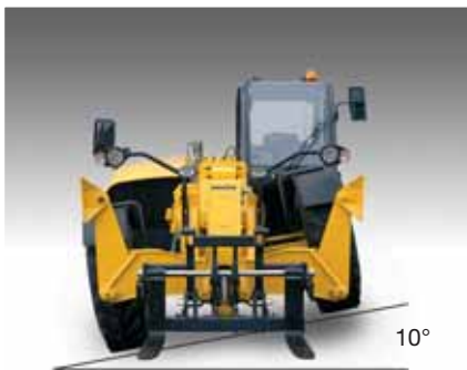
Frame levelling keeps the tool carriage horizontal, whatever the ground condition. It reaches angles of 10° on both sides and increases flexibility and lifting performances.
