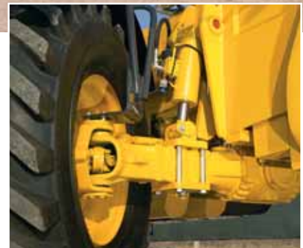
An automatic rear axle oscillation lock enlarges the bearing area, thus increasing both lift performance and security and reducing the risk of lateral tipping. It engages automatically over a 50° boom angle.
